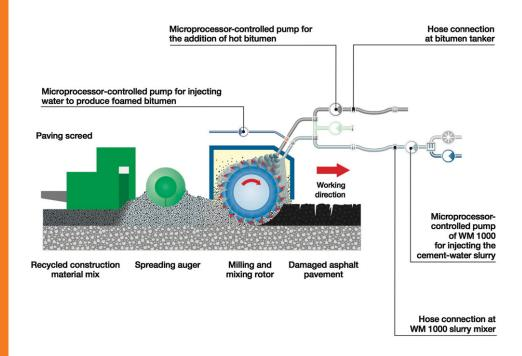
We use the Wirtgen Cold Recycler 3800CR for CIR jobs. This is a single unit train that pulverizes existing asphalt to a maximum depth of 6 inches, which is mixed with an asphalt binder and water in the machine's milling and mixing chamber to create a new mix. The mix is spread uniformly across the road.
